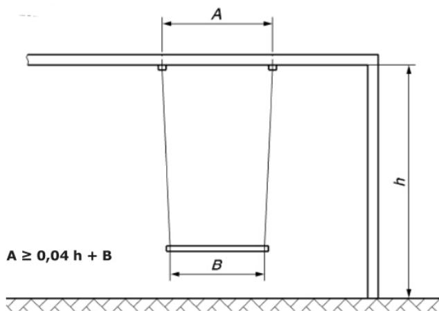
A - Distance between the suspension points along the crossbeam.
